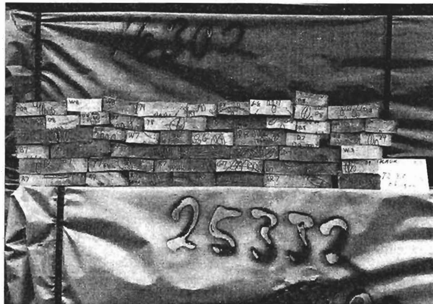
Photographic assessment of internal defects in boards after seasoning.
