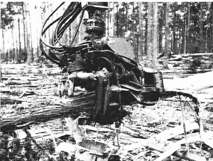
The modified Lako grapple harvester felling and debarking thinnings in a Tasmanian trial. The fibrous and voluminous bark is left on the forest floor, reducing the costs of transport and bark disposal at the mill and returning significant amounts of nutrients and organic matter to the site. The effect of increased fuel loadings on fire behaviour is not known.
